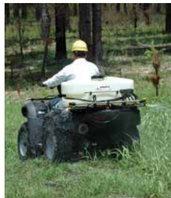
ATV mounted sprayer with a boom.
