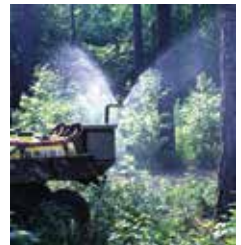
Spray pattern of two Boom Buster nozzles.
