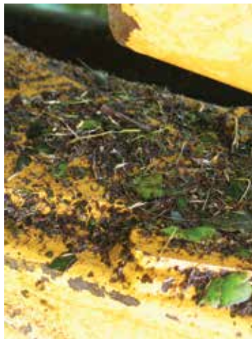
Excess grease traps seeds.
