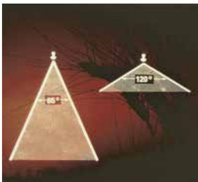
Nozzle spray angles of 65 and 120 degrees.
