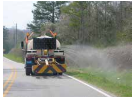
Roadside sprayers can treat invasives along highways.
