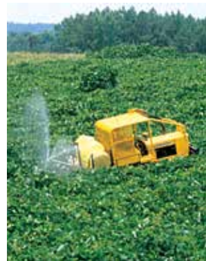
Boom Jet® nozzle on a crawler tractor spraying kudzu.
