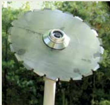
Brushsaw blade with chainsaw-like teeth.
