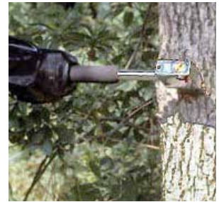
Hypo Hatchet® Tree Injector.
