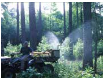
RTV mounted sprayer with Boom-Buster nozzles.
