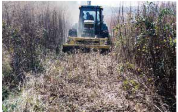
Wetblade brush mower applies herbicide while cutting.
