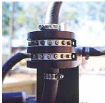
Radiarc® Sprayer 22-tip head.
