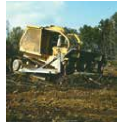
Brush rake attachment for a bulldozer.
