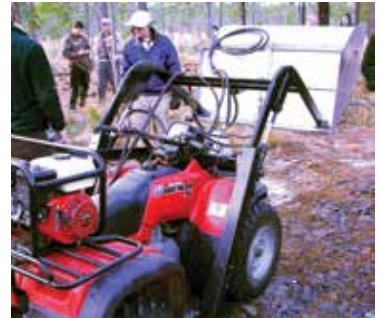
Grass seed harvester on an ATV.
