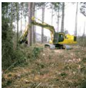
Boom-mounted mulcher head.
