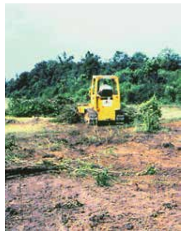
Bulldozer scrapes and piles Chinese privet.
